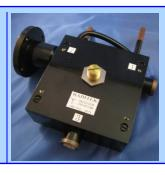
2.2 Kilo Watts Coaxial Circulator, 321.5-322.5MHz, 7/16 and 1 5/8 - Female Connectors, , Counter-Clockwise Rotation, Water Cooled For operating frequencies up to 1.0GHz coaxial isolators and circulators are available that can handle power up to 3500 watts with bandwidth up to 30% of the center frequency.
