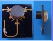
The devices should be mounted on the NON MAGNETIC carrier or base. The minimal thickness is 1.5mm. Plating: Gold, RoHS and REACH compliant. Load and Tuning conductor (97in3Ag). Optional location and configuration determined by vendor.
