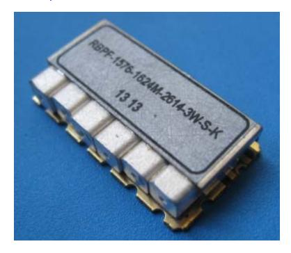
RADITEK's family of Model 2614, Surface Mount Ceramic Band Pass Filters are 26.4x14mm and operate in the frequency range of 980MHz to 6.54 GHz in Split Bands and in various bandwidths.
