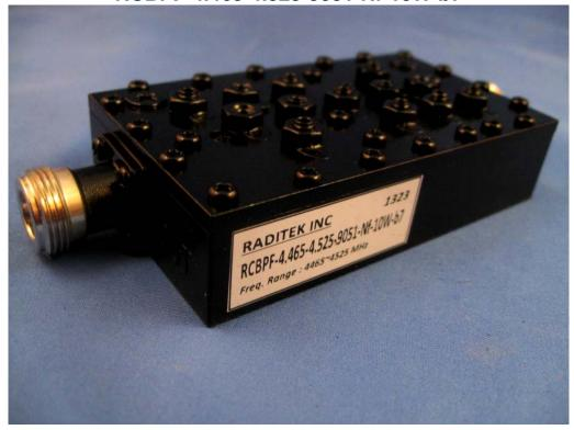
RADITEK's RCBPF-4.465-4.525-9051-Nf-10W-b7 Cavity Band Pass Filters a center frequency of 4495 GHz and an insertion loss of 1dB and a Return Loss of 14dB. It can handle 10 Watts of Power handling and the operating temperature of -10  $\sim$  +60°C. The Finish is Black Epoxy Paint and it has N-Type Female Connectors on all ports.
