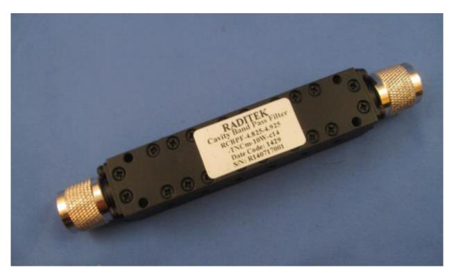
RADITEK'S RCBPF-4.825-4.925-TNCm-10W-c14 Cavity Band Pass Filters a center frequency of 4.875 GHz and an insertion loss of ≤1.5dB and a Return Loss of ≥15dB. It can handle 10 Watts of Power handling. The Finish is Black Paint and it has TNC Male or Female Connectors on all ports.
