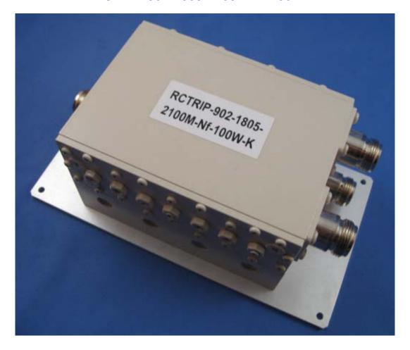
RADITEK's new Triplexer Features a Cavity Design, Low Loss and High Power Handling. Our newest model, RCTRIP-902-1805-2100M-Nf-100W-k, CH1 902~960MHz, CH2 1805~1880MHz and CH3 2110~2170MHz operate with an Insertion Loss of 0.5dB maximum and a Return Loss of 18dB minimum and 100 Watts of Input power with N-Type Female Connectors. Operating Temperature Range -20 to +70°C
