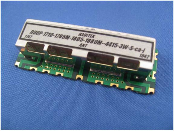
RADITEK'S DCS Band Surface Mount Ceramic Diplexer A high-performance DCS duplexer in a convenient surface mount package. Used mainly for splitting transmit and receive signals to and from a common antenna. RDUP-1710-1785-1805-1880M-4415-3W-S-ca-j Series typical performance specifications: 3dB Insertion Loss, 48dB Isolation / Rejection, 13dB Return Loss, -40 to +85°C Operating Temperature.
