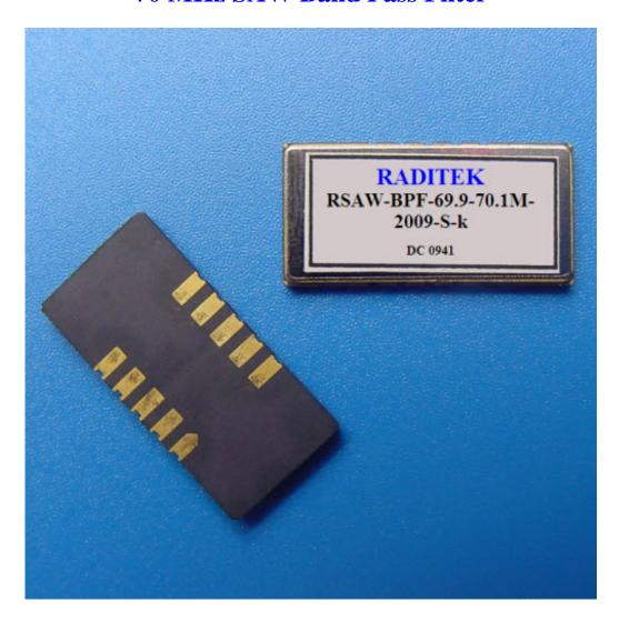
**RSAW-BPF 69.9-70.1MHz: RADITEK** specializes in Design, Development, Manufacturing of "High Volume/Low Cost" Wireless and Microwave products. Our new SAW Band Pass Filter operates at 70 MHz with a bandwidth of ±0.10. Insertion Loss: Fo 18.36 dB, Passband Ripple: 0.69 dB, 3dB Bandwidth: 3.608 MHz, Attenuation: 17.31dB @ Fo-2.1MHz and 20.62dB @ Fo+2.1MHz
