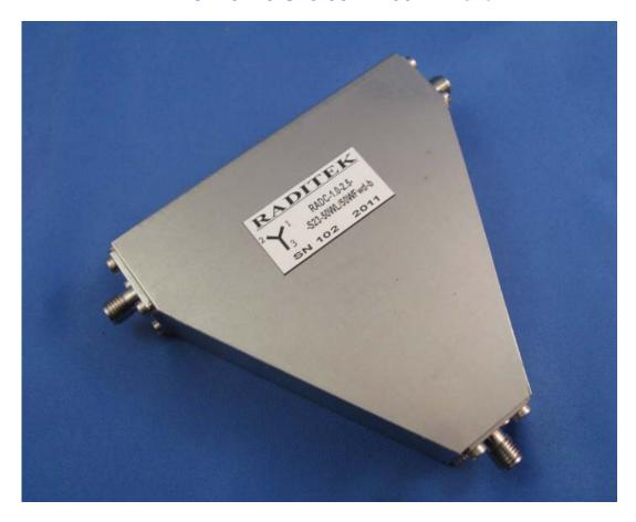
RADITEK'S Octave Plus Circulators are a cost effective solution for wide band frequency applications. This model covers 1.0-2.5 GHz with 50 Watts Average Forward and Reverse Power. Additional Reverse Power Options available are: 1, 5, 10, 20, 25 and 100 Watts Typical Specifications: 0.9dB Insertion Loss, 14dB Isolation, VSWR 1.55:1. Operating at Room Temperature. Dimensions: 78.8 (W) x 77.0 (L) x 21.2 (H) mm
