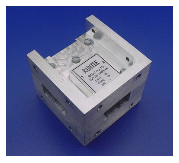
Our newest Waveguide Circulator, the RADC-10-15-WR75-2WR-4e, is a 10.0-15.0GHz waveguide circulator with WR75 flanges and 2 Watts or 600 Watts of power handling with dimensions of 44.5 X 44.5 millimeters. This series can actually handle any frequency from 10-15GHz with 10% operational bandwidth standard, with wider bandwidth versions available upon request. Operating over the full temperature range of –30 to +70°C, specifications are insertion loss 0.2dB, isolation 20dB, and VSWR 1.22:1 maximum.
