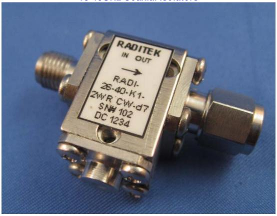
RADITEK's newest Coaxial Isolator Family spans 18 to 40GHz using K/2.9. The part pictured RADI-26-40-K1-2WR CW-d7, is a 26-40GHz coaxial isolator with K/2.9mm connectors and 2Watts of continuous power handling. Operating over the full temperature range of -20 to +65°C. Specifications: Insertion Loss 1.0dB maximum, Isolation 14dB minimum, and VSWR 1.50:1 maximum. Dimensions without connectors: 0.50 x 0.85 x 0.50mm. Dimensions with connectors: 1.382 x 0.85 x 0.50mm.
