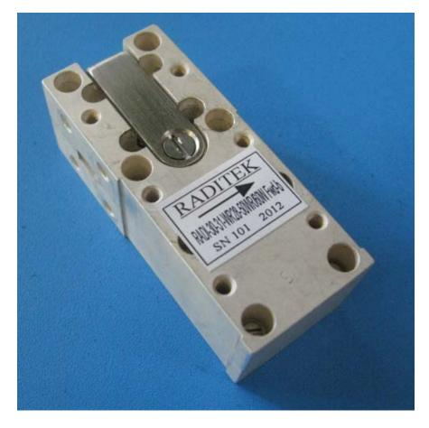
RADITEK's latest 29-31.5GHz Ka Band High Power Waveguide Isolator operates at 60Watts of Forward and 50Watts Reverse Power and has a new compact design, 23x63x25.4mm, with a WR28 waveguide flange. General Specifications for model shown: Insertion loss(0.4dB), Isolation(20dB), VSWR(1.25:1).Operating Temperature: -35~+55\*C Device should be mounted on the heatsink and the surface temperature should not be higher
