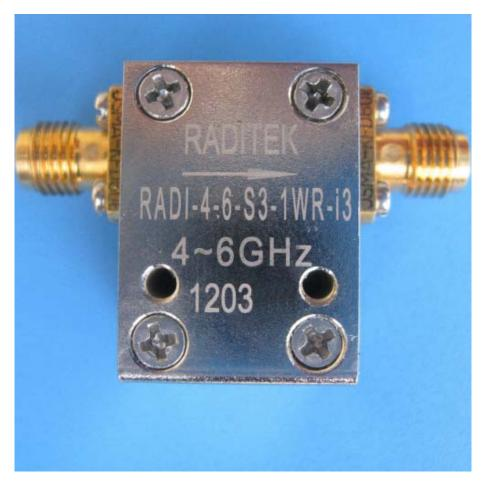
RADITEK'S new Wide Band Isolator operates at 4-6GHz Full Band and 1 to 50 Watts of Power. SMA Female Connectors are standard and a new compact design of 17x14x23mm. General Specifications for model shown: Insertion loss (0.4dB), Isolation (20dB min), VSWR(1.25:1).Operating Temperature: -20~+70\*C These units are proven in the field and are fully ROHS compliant.
