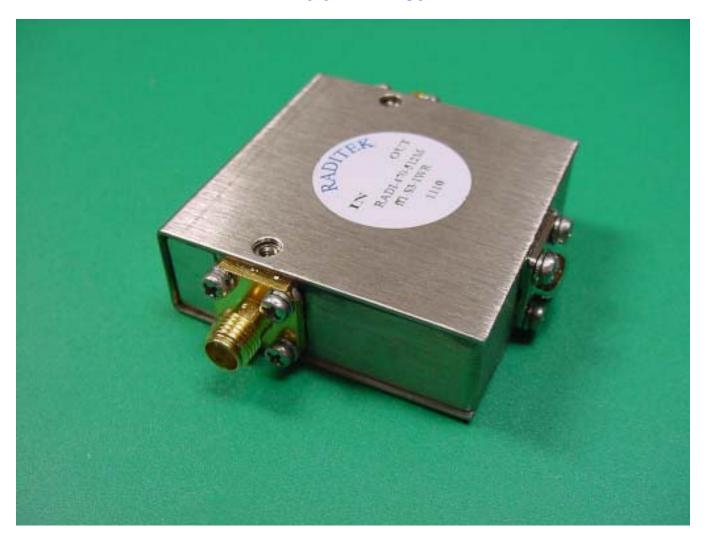
RADITEK'S Our newest Coaxial model, the FF1 Series, is a 360-540MHz, 10% Bandwidth Isolator and Circulator with 100 watts forward and 10 watts reverse power handling typical. Operating over the full temperature range of 20 to +85°C. Specifications over temperature are 0.4dB insertion loss, 22dB isolation, and 1.2:1 VSWR maximum. Dimensions: 44.45 x 45.47 x 15.75 millimeters
