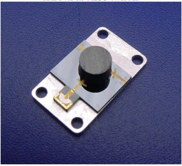
Microstrip MSSC Series Isolator, Our newest model, the MSSC series has a small compact size with the extra mounting flexibility of the steel back and mounting and 5Watts reverse power maximum due load size and hole spacing. They operate in the range between 5.6-26.5GHz and sizes vary by frequency. Specifications over full operating temperature (-40 to +70 °C), Survives, non-operating 130 °C for up to 2 hrs.
