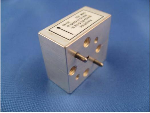
*RADITEK's* 89.5-94.5GHz, WR10 Waveguide Isolator used in scientific research and intra campus high data rate communications. The standard units are ultra low loss with a silver plated brass construction. Specifications: <0.5 dB Insertion Loss, >18dB Isolation, <1.70:1 VSWR Dimensions (mm): 12(W) x 25(H) 22(T).
