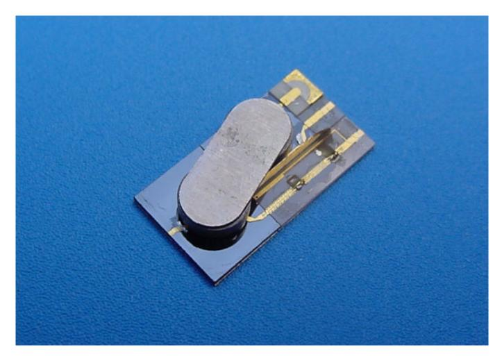
Microstrip Duplexer with Limiter 9.2-10 GHz Dual Junction, RADITEK specializes in Design, Development, Manufacturing of "High Volume/Low Cost" Wireless and Microwave products. Our New Microstrip Duplexer (Circulator/ Isolator) with Limiter, RCI-LIM-A-9.2-10.0-MSDJ-10/10W-e, operates at 9.2-10.0GHz with 10 Watts power. Isolation: Antenna to
