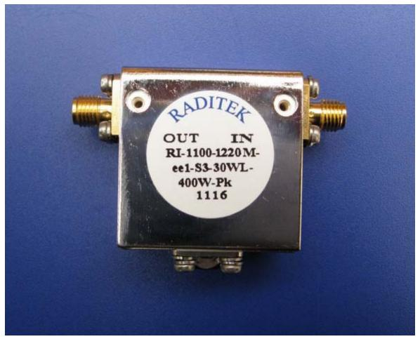
RADITEK's new ee1 Series coaxial Isolators are the most economic for PCS, Cellular, DMB, and Wi-Max applications. These cover the full band of 640MHz-2.5GHz at 10% Bandwidth over -20 to +85 degrees C. SMA or N-Type Connectors available. It has better than 20 dB return loss and 21 dB isolation, and can handle 120W forward and 35W reverse power and up to 500W peak power. Circulators also available.
