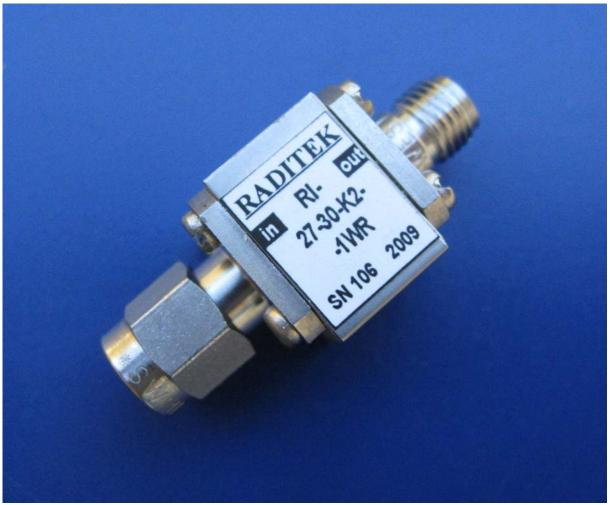
Our newest Coaxial Isolator Family spans 17 to 45GHz with up to 3GHz bandwidth using either K/2.9 or 2.4 connectors. The part pictured, RADI-27-30-K2-1W, is a 27-30GHz coaxial isolator with K-Type connectors and 1 watt of power handling. Specifications: 1.1 dB Insertion Loss, 20dB Isolation, 1.35:1 VSWR, -30 to +65°C Operating Temperature,
