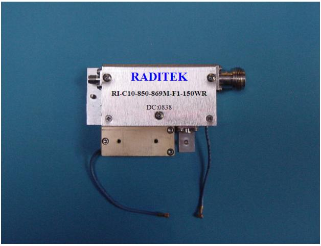
This Robust, high power, double junction Cellular Band 850-869MHz Coaxial Isolator: spectacular 65dB Isolation, (typically > 70dB). 0.45dB insertion loss, 1.20 VSWR, SMAf on input, Nf on output with input and output monitor cables. 150Watts Reverse Power, 200Watts Forward Power and 1500Watts Peak Power. These units are proven in the field and are fully ROHS compliant.
