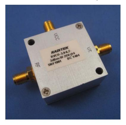
RADITEK'S Voltage Controlled Oscillator, RVCO-3.9-6.7-2dBm-SF-25V-j14, operates in the frequency range of 3.9-6.7GHz with -2dBm of Output Power and a Tuning Voltage of 0.5-18 VDC. Fitted with standard SMA Female connectors.
