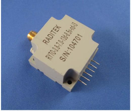
Raditek's Mini-Ylg oscillator. Our customers requested this product to replace discontinued models from other companies. We responded by adding the first two frequency bands, 3.8-7GHz and 3.95 to 9GHz and creating a matching Mini YlG family of oscillators.
