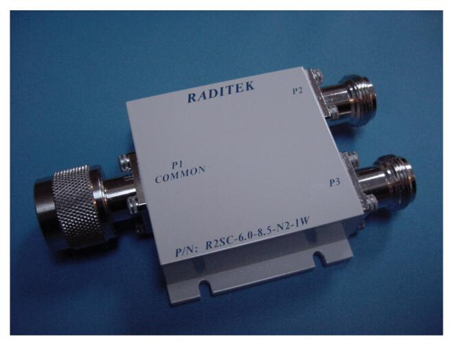
RADITEK'S Our new weatherproof 2 way Splitter Combiner is designed to connect directly into a mast top Antenna to allow connection of two Transceivers. These can be equally split or at a 3:1 ratio with 2.5dB insertion loss on the low loss port, optimizing the main unit while permitting a standby to monitor.
