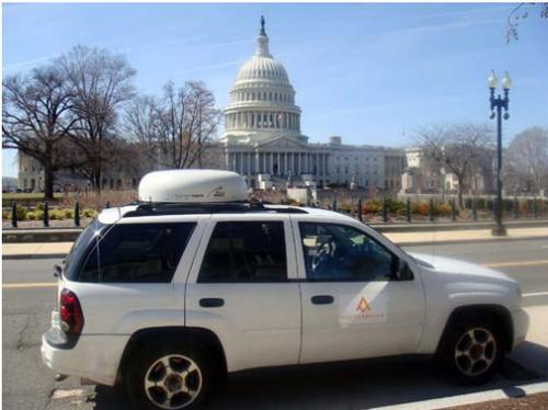
The IOTM-Ku- fits on a standard roof rack. Low profile, small footprint..
