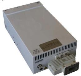
Complementing the other RADITEK super-efficient, smaller size, lighter and more powerful BUC series. This model offers significant higher power BUC size and weight reduction and at the same time substantially improves thermal efficiency, which leads to higher reliability and longer MTBF.
