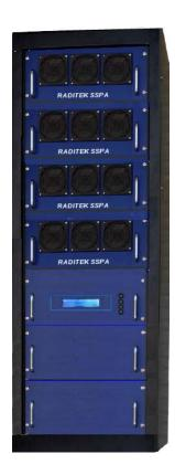
The PSUs (Power Supply Units) are also hot swappable, consisting of 8 PSUs, each delivering 2KW of DC Power. All of the PSUs are constantly monitored, and all critical data is available via internet (read only) or by interactive RS232//USB link locally.
