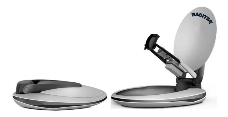
RADITEK'S RANT-Ku or C-2.4M-Rx-Tx-VMA-x15 is a complete 2.4m carbon fiber reflector based, tracking transmit and receive, vehicle mount antenna for C and Ku band. It can transmit to 300W, and has linear polarization skew adjustment as well as Az and El actuators. The unit has a self contained ACU (Antenna Control Unit) with processor, motor drivers, GPS compass, and control.
