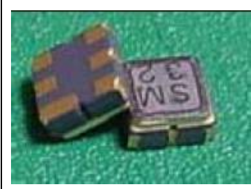
Saw Filters, GSM PCS Etc SMT 3mm square excellent for cell phone use and many other applications. very sharp slope responses
