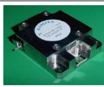
Stripline Isolator's and Circulators 400 MHz 100W
