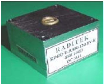
DRO, PLDRO EXTERNAL and INTERNAL Reference, 1 - 42GHz
